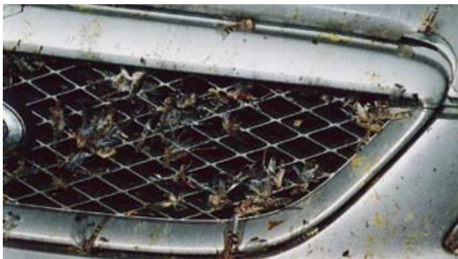
Locust damage to radiator
